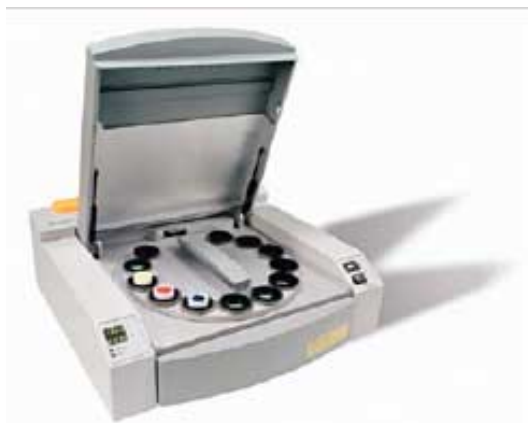
Fig. 4 Compact energy-dispersive X-ray fluorescence spectrometer.
